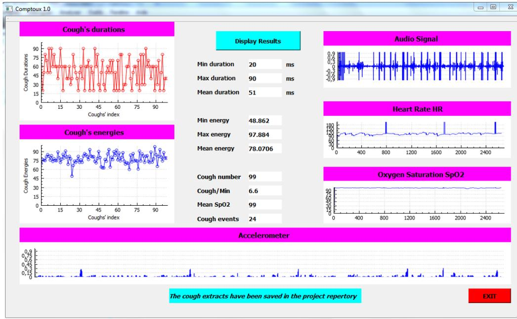
Fig. 4: *Sensor-based Interface for Automatic Cough Detection.*
