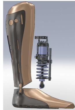
Fig. 9: The orthosis prototype is composed of several main components. The spring is used to stock energy during specific gait phases. A homemade ultra-compact actuator of around 3 kg is controlling the orthosis in a way depending on the current gait phase. Moreover, this system is suitable for an active stance phase as well.
