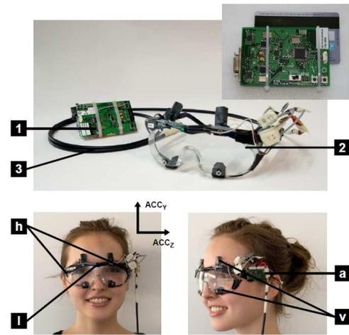
Fig. 2: There are several components in the EOG-based wearable eye tracker: the DSP (1), the Goggles (2) and the shielded core cable (3). The pictures at the bottom show the Goggles worn by a person with the positions of the two horizontal (h) and vertical (v) dry electrodes, the light sensor (l) and the accelerometer (a) with direction of its axes (ACC\_Y, ACC\_Z). [33]
