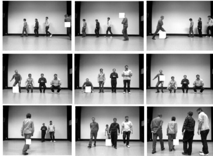
Fig 7: Speed scenarios along 3 axes. The white blobs locate the person which has different speed on the X axis (first row), on the Y axis (second row) and on the Z axis (third row).
