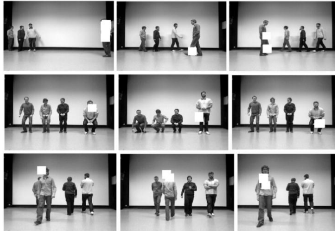
Fig 6: Direction scenarios along 3 axes. The white blobs locate the person which has different direction on the X axis (first row), on the Y axis (second row) and on the Z axis (third row).
