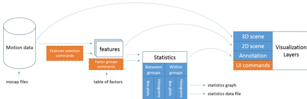
Figure 1 – Factor Statistical exploration module general block diagram
