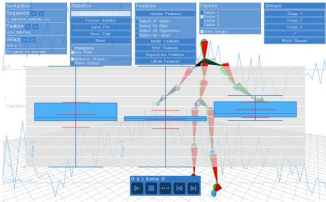
**Figure 2 - Interface of the statistical exploration module. The four visualization layers are activated. First, the 3D scene displays the ground (gray grid) and the 3D skeleton at a given frame of a sequence. Secondly, the 2D figure scene displays continuous motion features (blue curves). Then, the third layer displays the box plots, and finally, graphical commands are displayed above all previous layers.**
