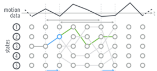
Figure 4: Real-time Viterbi decoding: the sliding window approach, i.e. decoding on a subpath and validation of the oldest state as decoded.
