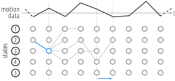
Figure 5: Real-time Viterbi decoding: the state stability approach, i.e. monitoring of past states variations and validation upon stabilisation.
