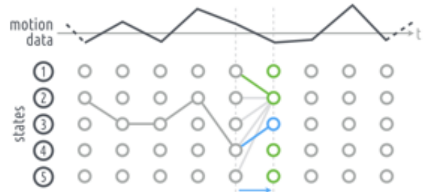
Figure 3: Real-time Viterbi decoding: the forward only approach, i.e. decision taken at each state.
