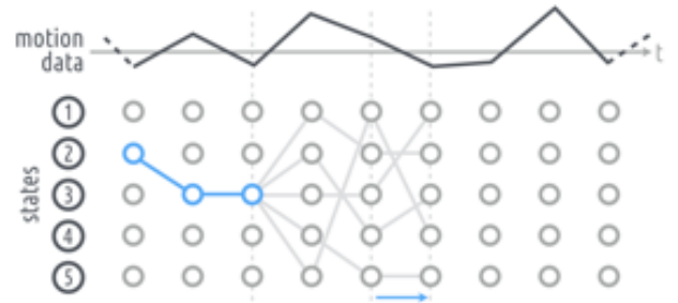
Figure 6: Real-time Viterbi decoding: the fusion point approach as described by Bloit and Rodet [2].
