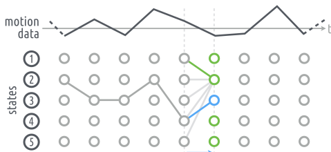
Figure 4. Realtime Viterbi decoding: illustration of the forward-only approach on a simplified five-state model. The “best” state sequence is determined for each increment in the Viterbi lattice.
