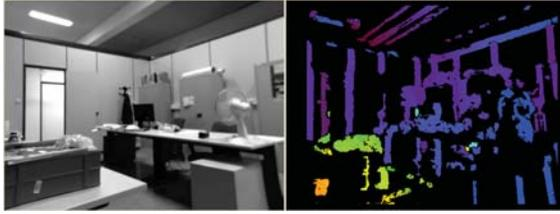
**Figure 2.** a. Left image of our stereoscopic camera. b. Depth map: orange shows a short distance to the camera.
