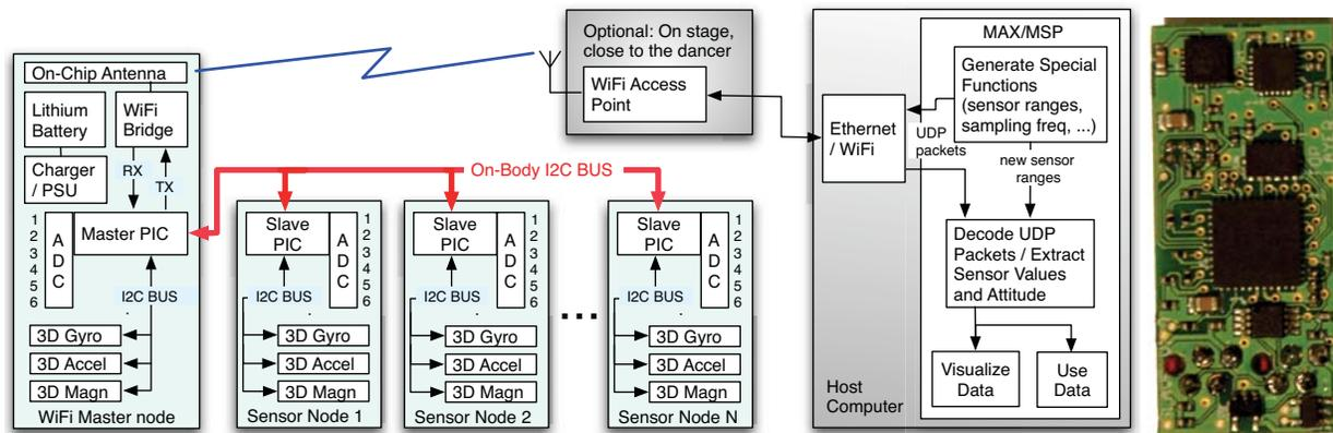
Figure 5. Left: Wireless sensor system global architecture, with all transmission paths (network, wireless, serial, local and on-body I2C, analog). Right: 17x38mm sensor node (connectors are located on the back).
