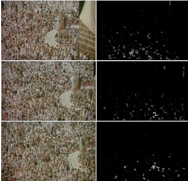
Fig. 6. Left image: original frame; Right image: global results: camera translation has very little influence on the algorithm results.
