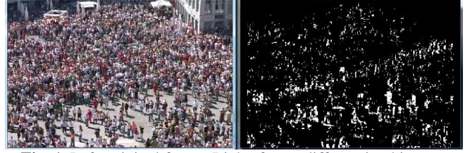
Fig. 1. Left: original frame; Right: frame-differencing history.
