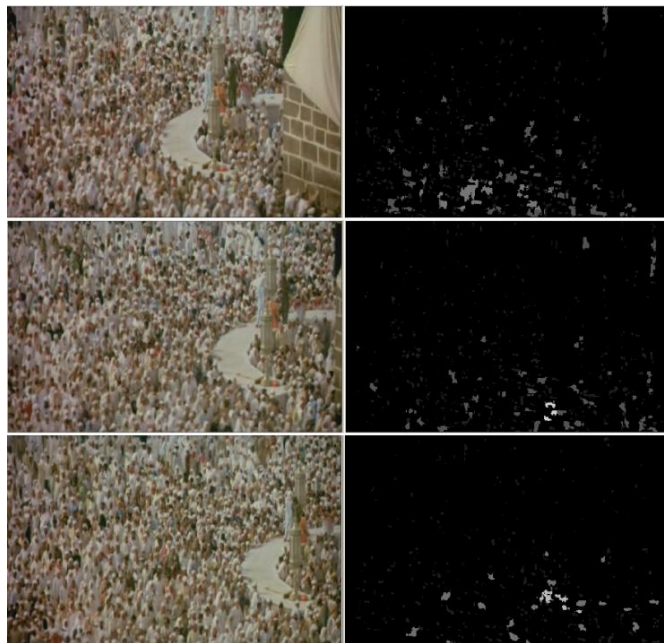
Fig. 7. Left: original frames with global translation; Right: global translation results: camera translation has little influence.
