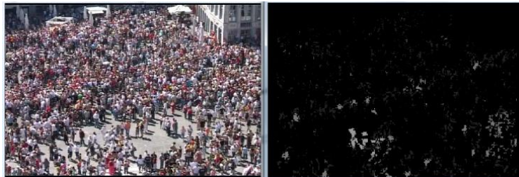
Fig. 4. Left image: original frame; Right image: global result: clear areas have a higher saliency index than the darker ones.
