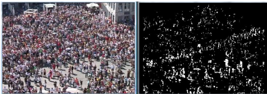
Fig. 1. Left: original frame; Right: frame-differencing history.
