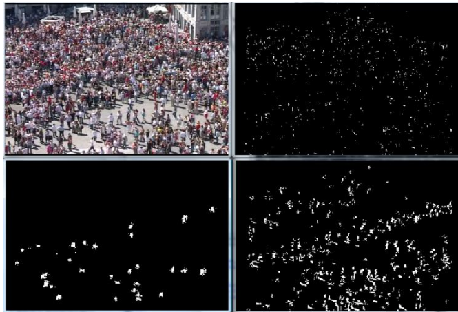
Fig. 2. Top-Left: original frame; Top-Right: small blobs (low-speed); Bottom-Right: medium blobs (medium-speed), Bottom-Left: large blobs (high-speed).
