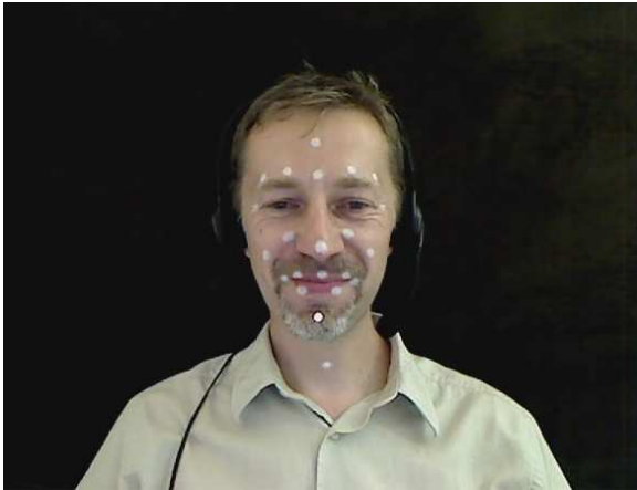
Figure 1: Markers drawn for facial motion tracking using ZignTrack
