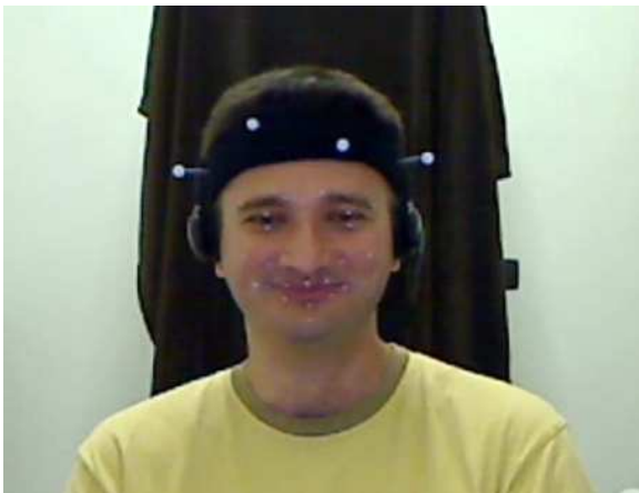
Figure 2: Infrared markers placed for facial motion tracking using OptiTrack
