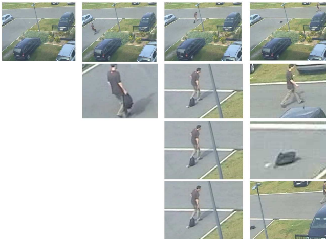
Fig. 7. New "zoomed versions" of video stream. First row is the original video stream. Second row is created when a first mobile object appears in the scene. Third row is created when a second object is detected and tracked (the abandoned luggage). Forth row is the stream that includes the two mobile objects.
