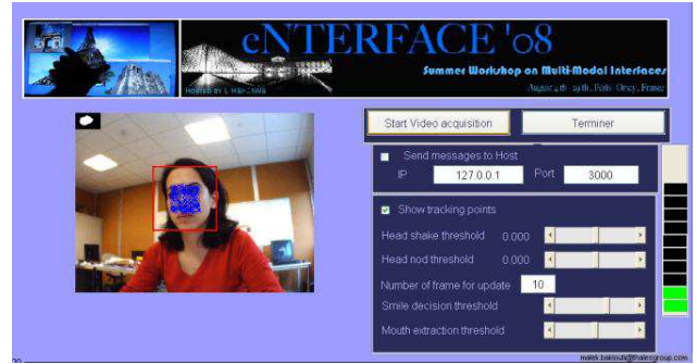
Fig. 4. Screenshot of the face analysis component, which runs on a PC and shows the analysis results through a MATLAB-based user interface. It sends its results to the multimodal fusion module via TCP-IP.
