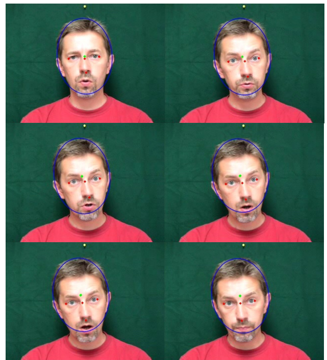
Fig. 12 Results of the global head movements tracking .The ellipse and the green point are the results of last year, red points is the new tracking method.
