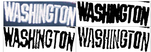
Figure 2. Original image (top left), binary version (top right), segmentation with large bandwidth (bottom left), segmentation with narrow bandwidth (bottom right)
