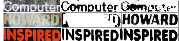
Fig. 2. Left: initial color images, middle: extraction done by D_{eucl} , right: extraction done by S_{cos} .
