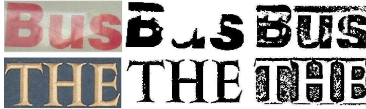
Figure 2. Applying Otsu (middle) or Sauvola (right) thresholding on original images (left) is a major decision at this point: top: the background is complex, Sauvola is the best algorithm, bottom: the background is clean, Otsu is the best algorithm
