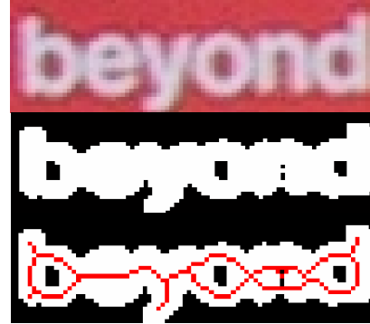
Figure 5: In top-down order: initial image, the mask M, M and its skeleton.
