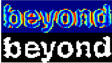
Figure 7: In top-down order: PhaseResult multiplied by the mask M , final result after Otsu-based thresholding.
