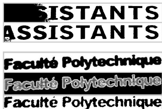
Figure 5. Top: the first image is got after Otsu thresholding and the second one after our binarisation. Bottom: the first image is the thresholded reconstructed image, the second one is the result of skeletonization on the image and the third one is the result with the new threshold for thick characters.
