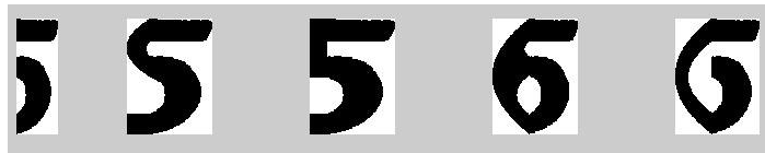
Figure 5. Possible prolongations of a cut character (on the left). This character is more probably a "5", but it could be a "S", a "6", or a "G".
