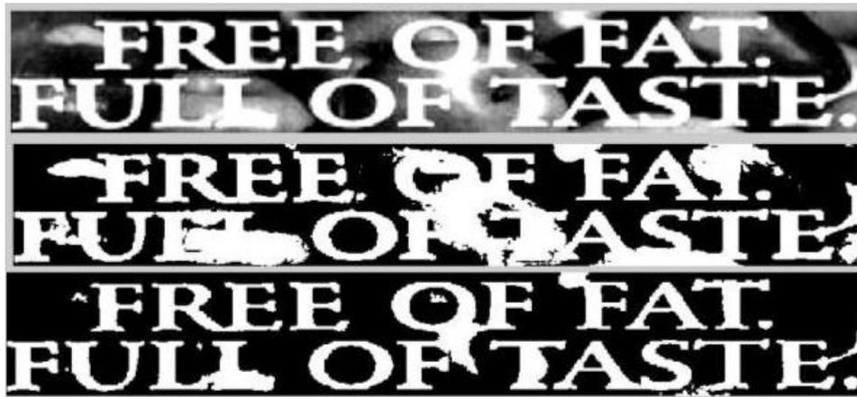
FIG. 3 – Improvement by re-applying the Otsu thresholding. From top to bottom : the reconstructed image, the thresholding on the reconstructed image and the iterative thresholding on the mask
