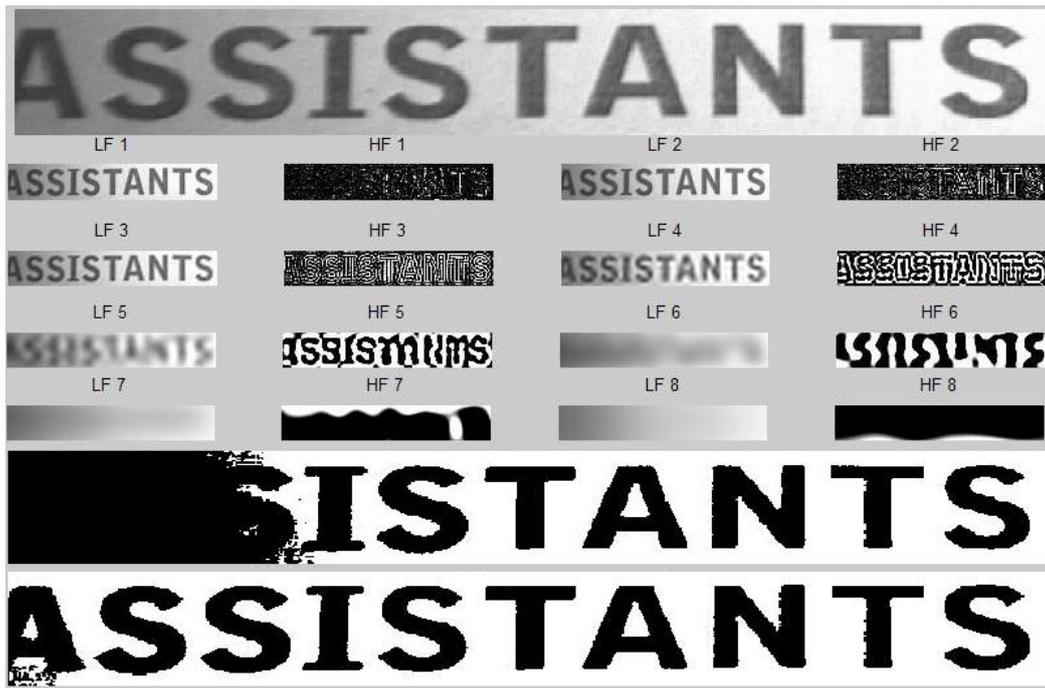
FIG. 1 – From top to bottom : the original image, the wavelet decomposition with multiple subimages, the thresholding on the initial image and the thresholding on the reconstructed image
