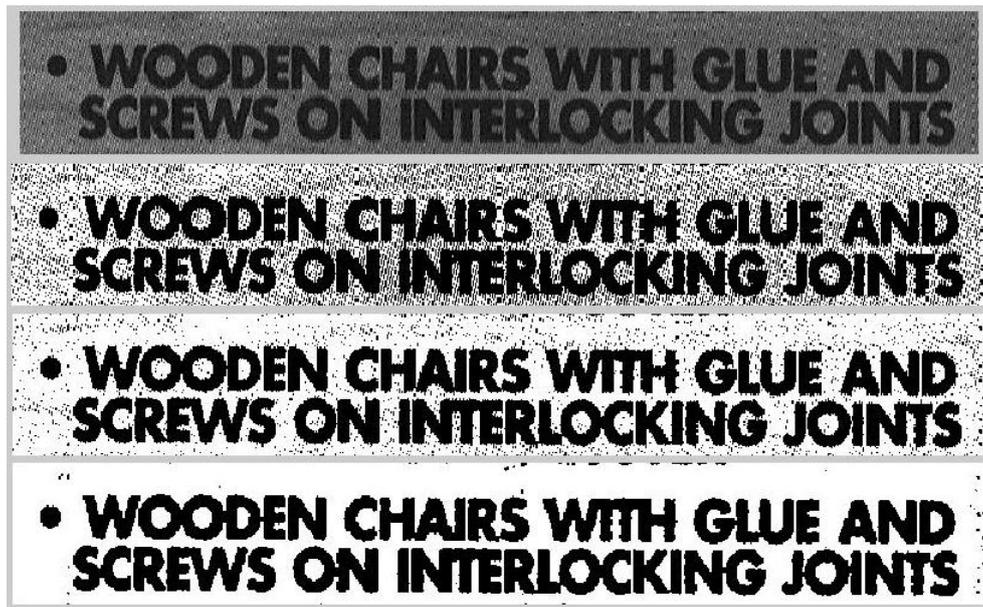
FIG. 4 – To remove salt and pepper noise. From top to bottom : the initial image, the binarized initial image, the binarized reconstructed image and the same one without HF1
