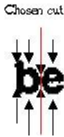
Fig. 8. Caliper algorithm: the chosen cut between 'b' and 'e'
