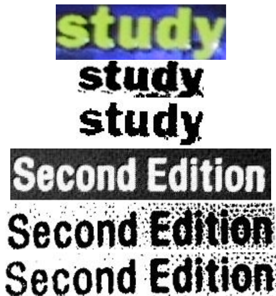
Fig. 6. From top to bottom: original RGB image, Otsu thresholding and our thresholding algorithm
