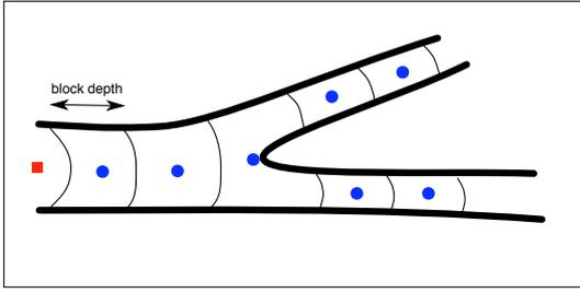
Fig. 2. The concept of *slices*. Seed voxel is represented as a red square, and successive centers of gravity as blue disks
