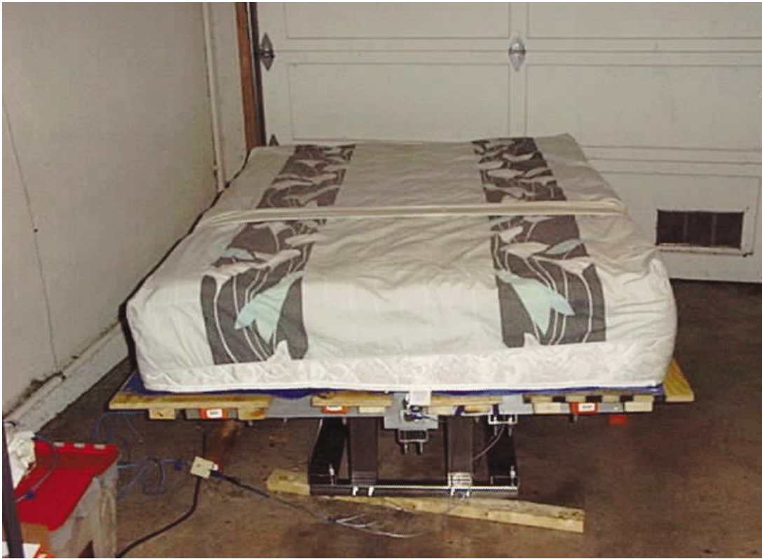
Figure 15. Morpheus bed with mattress, showing also the transverse mattress sensor belt placed under the torso of the sleeper.
