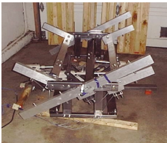
Figure 13. Bed frame with wooden segments removed to show subframe assemblies.
